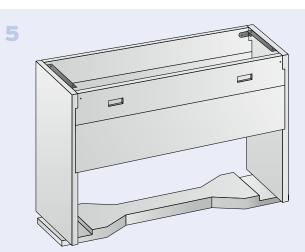
From the front panel, which consists of two parts, first attach the larger panel at the bottom with screws and brackets. To attach the upper front panel (version removable from the outside), the brackets must first be screwed to the side panels. The chain must be attached with the spring cotter pin through the screw. Then pull the two sliding nuts over the angles. Next, fasten the upper front plate from the outside using the hexagon socket screws.
