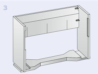
From the rear panel, which consists of two parts, first connect the larger panel at the bottom and then the smaller panel at the top to the side panels using two screws and brackets each. The larger panel - with cast-in anchor rails - is used to hold the cable retaining rail.
